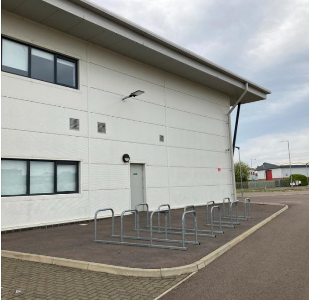
Cycle parking at a commercial building. The cycle parking is not covered and there isn't a dropped kerb to enable cyclists to access the cycle parking. Without a gated entrance to the premises and no additional security, bikes could be vulnerable to theft.
