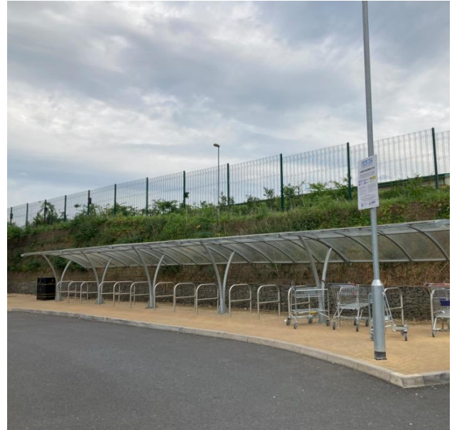
Cycle parking at a retail park. There is no dropped kerb for cyclists to access the cycle parking, and its location in the top corner of the car park is not convenient when there are many parking spaces that are closer to each retail unit. There is no additional layer of security for long-term cycle parking.
